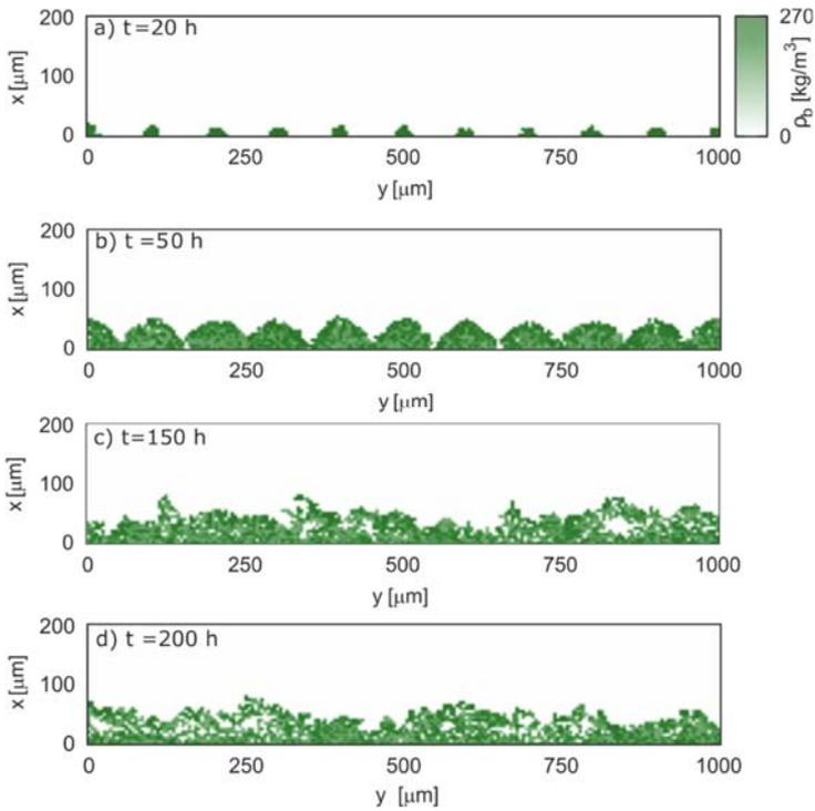
Fig. 6. Two-dimensional distribution of the biofilm density dependent on time:
