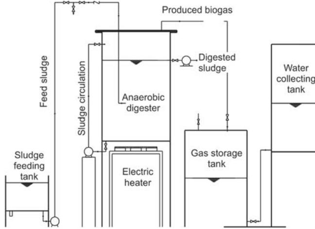
Fig. 1. Schematic illustration of the experimental test rig
