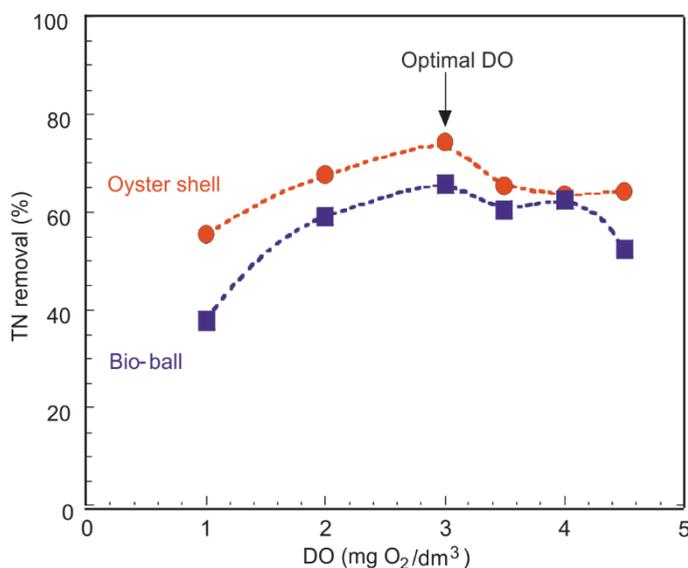
Fig. 3. Determination of optimal DO for the filters
