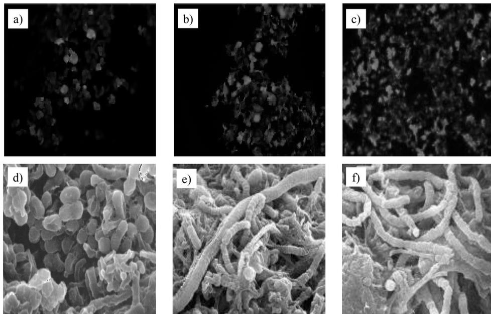
Fig. 6. FISH and SEM images of activated sludge in seed sludge and at the end of acclimatization period: a) seed sludge, PAO (9.3%) + DAPI, 50 $\times$ , b) AA sludge, DPAO (61.6%) + DAPI, 50 $\times$ , c) AO sludge, PAO (79.3%) + DAPI, 50 $\times$ , d) seed sludge, 5000 $\times$ , e) AA sludge, 5000 $\times$ , f) AO sludge, 5000 $\times$
