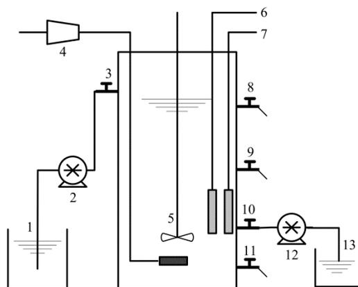
Fig. 1 Schematic diagram of experimental setup: 1 – influent tank, 2 – influent pump, 3 – water inlet, 4 – air pump, 5 – mixer, 6 – ORP/pH meter, 7 – DO meter, 8, 9 – sample points, 10 – water outlet, 11 – waste sludge outlet, 12 – effluent pump, 13 – effluent tank
