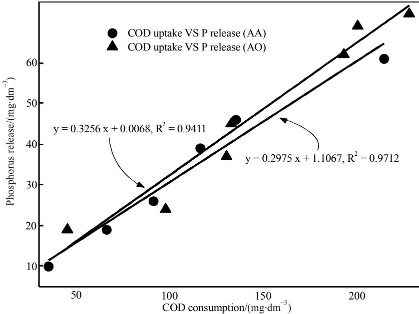
Fig. 3. Dependences of phosphorus release on COD uptake for AA and AO sludge in anaerobic conditions
