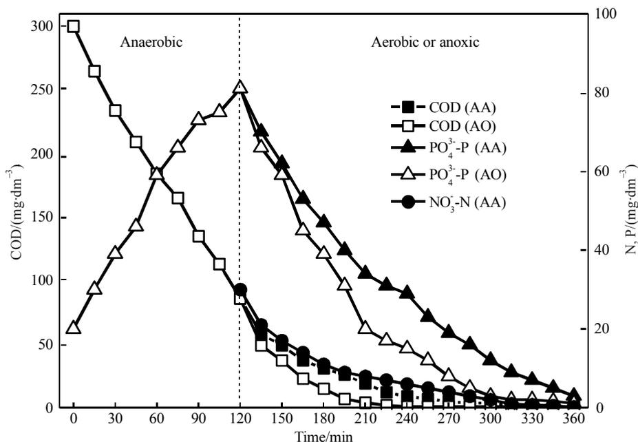
Fig. 4. Carbon, nitrogen and phosphorus profiles of DPAO sludge exposed to anaerobic-aerobic or anoxic conditions
