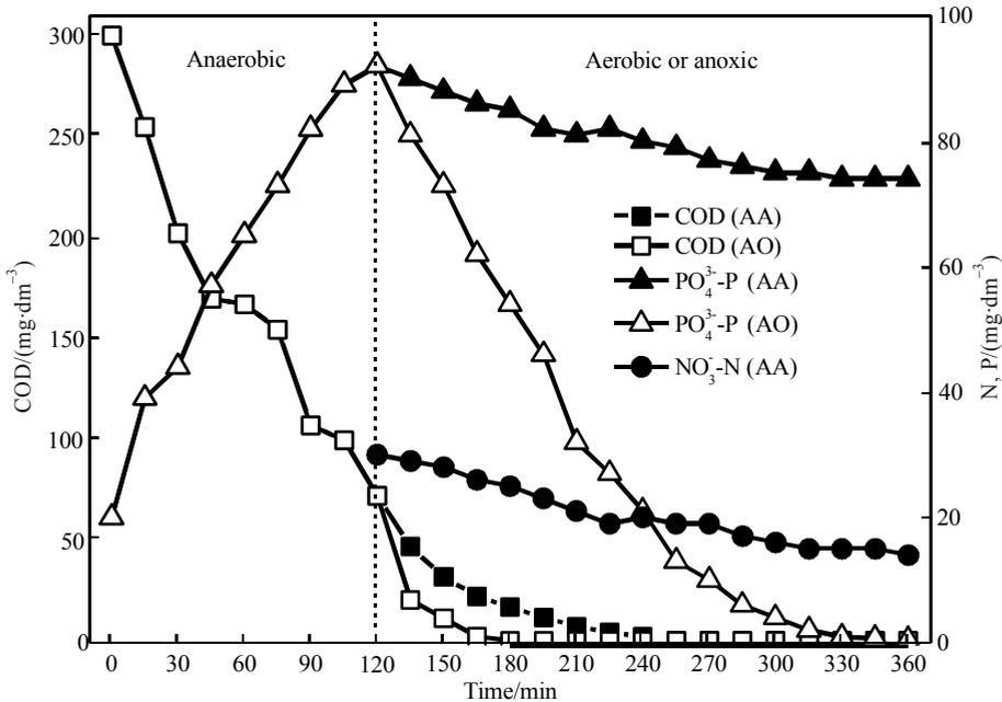
Fig. 5. Carbon, nitrogen and phosphorus profiles of PAO sludge exposed to anaerobic-aerobic or anoxic conditions
