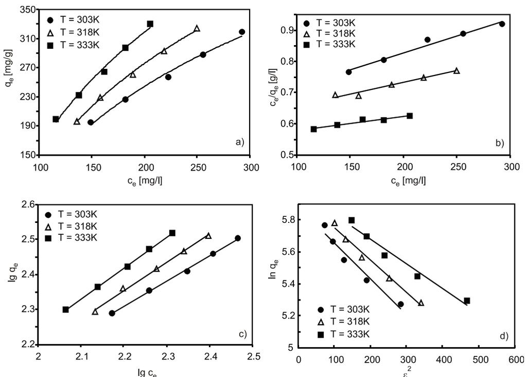
Fig. 7. Equilibrium isotherm of OPs-CW adsorption onto MCFA ( $T = 303$  K,  $t = 10$  h, MCFA dosage = 2 g/l, pH = 6.0): a) equilibrium adsorption isotherm, b) Langmuir model, c) Freundlich model, d) D-R model
