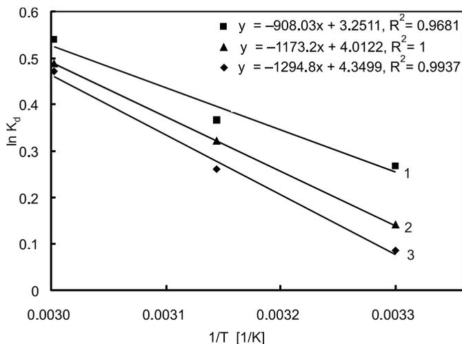
Fig. 9. The plot of  $\ln k_d$  vs.  $1/T$  at initial COD concentrations of 355 (1), 712 (2), and 2845 (3) mg/l of coking wastewater
