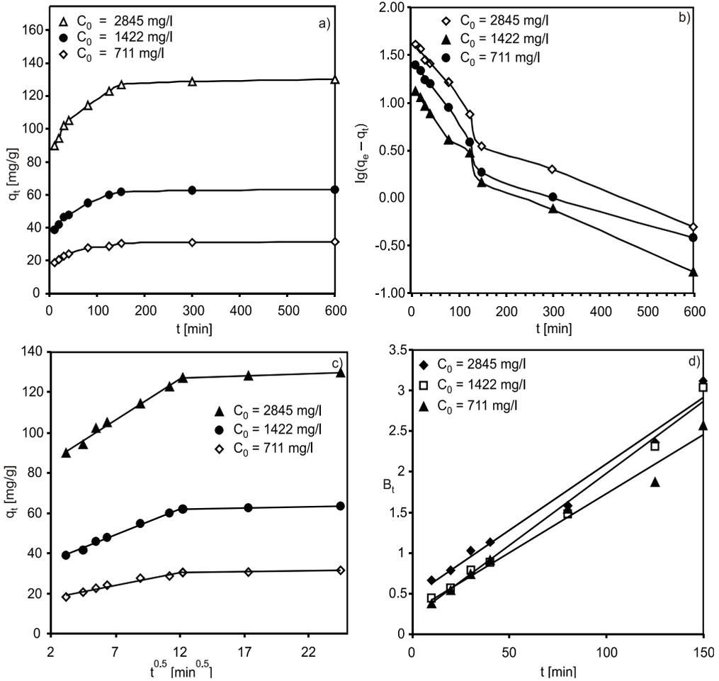
Fig. 6. Kinetics of OPs-CW adsorption onto MCFA ( $T = 303$  K,  $t = 10$  h, MCFA dosage = 2.0 g/l, pH = 6.0): a) effect of contact time, b) plot of pseudo-first order model, c) plot of Weber and Morris model, d) plot of Dumwald–Wagner model
