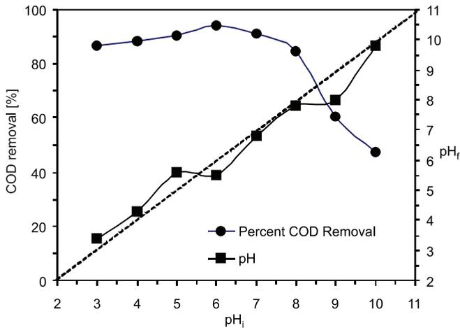
Fig. 5. Effect of initial pH on the OPs-CW adsorption by MCFA ( $T = 303 \text{ K}$ , contact time – 12 h,  $C_0 = 2845 \text{ mg/l}$ , MCFA dosage = 2.0 g/l)
