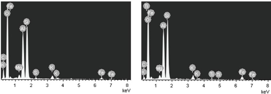
Fig. 2. Surface elements profile of RCFA (a) and MCFA (b)
