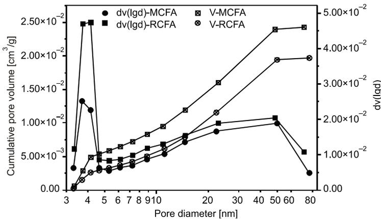
Fig. 3. Pore size distribution of RCFA and MCFA
