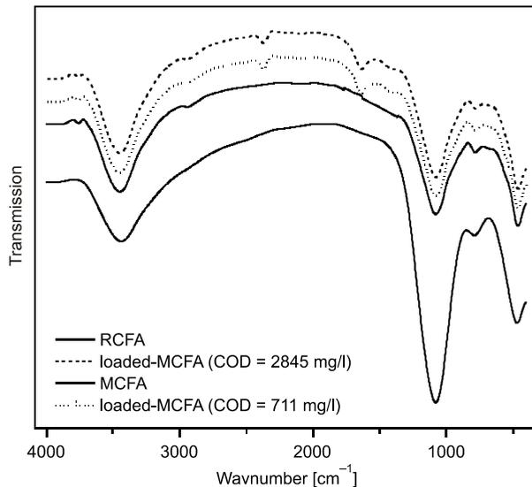
Fig. 8. FT-IR spectrogram of blank RCFA, MCFA and OPs-CW loaded MCFA
