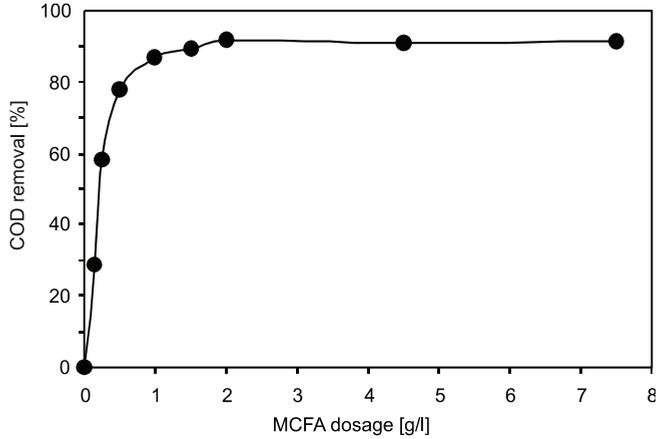
Fig. 4. Effect of MCFA dosage on OPs-CW adsorption onto MCFA ( $T = 303 \text{ K}$ ,  $t = 10 \text{ h}$ ,  $C_0 = 2845 \text{ mg/l}$ ,  $\text{pH} = 7.0$ )
