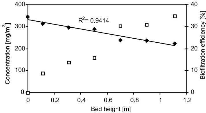
Fig. 5. Biofiltration performance of MIBK on biological bed with pine bark and compost (2:1 v/v ratio) at high concentration of the additive: diamonds – MIBK concentration in the air, squares – biofiltration efficiency; inlet concentration 344.5 mg/m<sup>3</sup>
