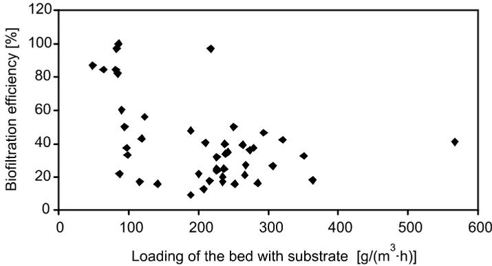
Fig. 2. Dependence of the biofiltration efficiency on the mass loading of the bed
