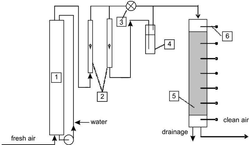
Fig. 1. Scheme of the experimental set up: 1 – humidifying column, 2 – rotameters, 3 – control valve, 4 – scrubber with tested substance (MIBK, 5 – biofiltration column, 6 – sampling ports
