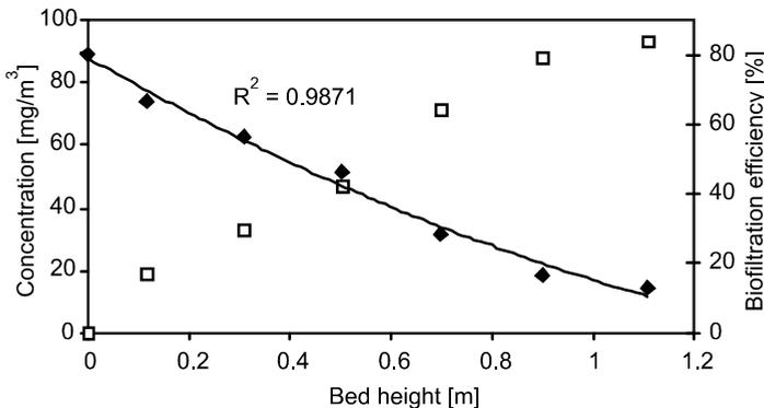
Fig. 4. Biofiltration performance of MIBK on biological bed with pine bark and compost (2:1 v/v ratio) at low concentration of the additive: diamonds – MIBK concentration in the air, squares – biofiltration efficiency; inlet concentration  $80.2 \text{ mg}/\text{m}^3$
