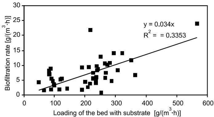
Fig. 3. Dependence of the biodegradation rate on the mass loading of the bed
