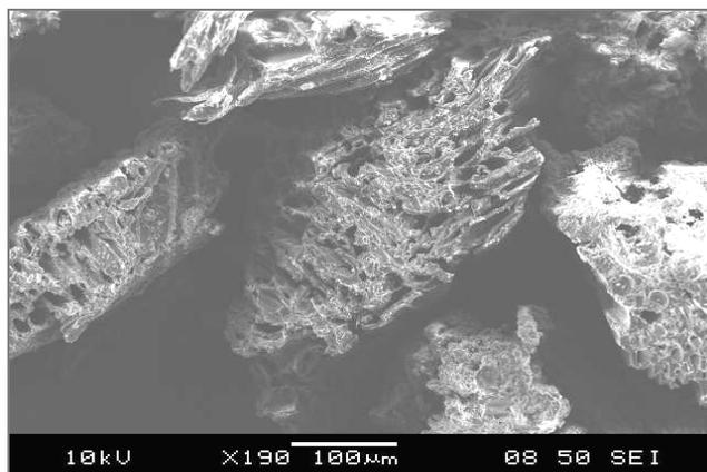
Fig. 1. SEM of the RCP carbon
