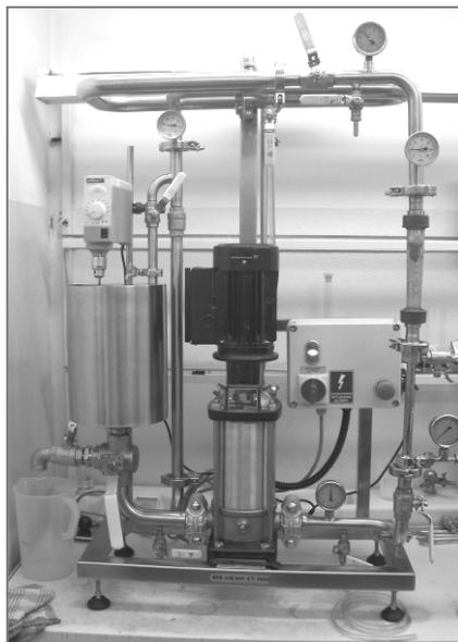
Fig. 1. Ultrafiltration cross-flow system
