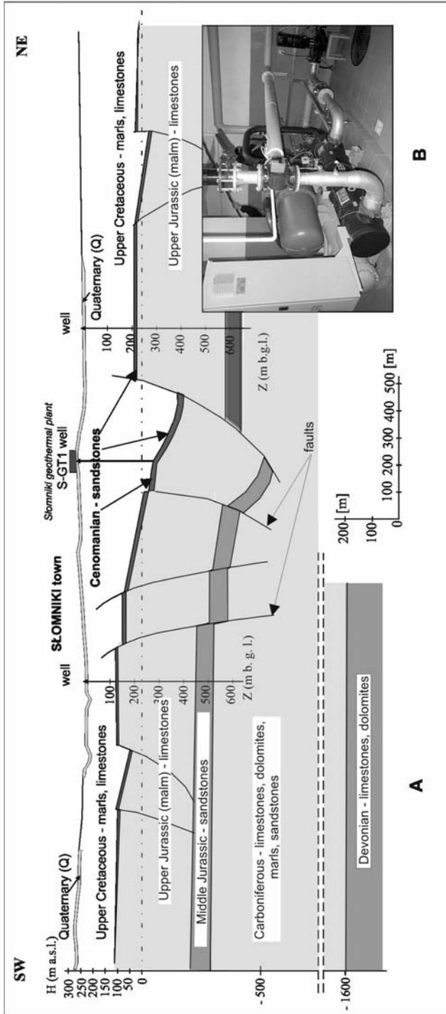
Fig. 2. Geological cross-section across the Miechów Trough near Słomniki (A) (location in figure 1). Compression heat pump (Ochsner, 320 kW) in Słomniki geothermal plant (B)
