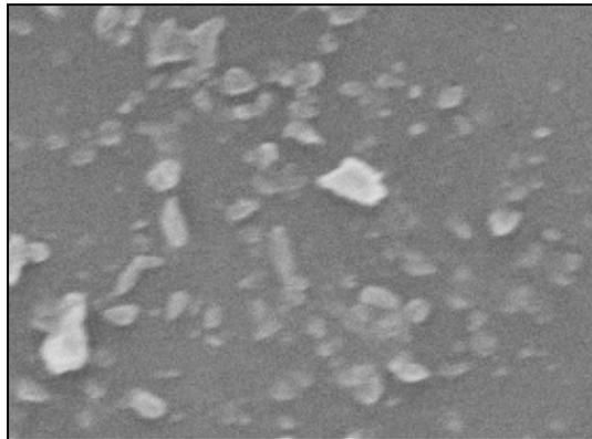
Fig. 4. SEM image of surface of new pipeline made of PP (magnification of 6 000×)
