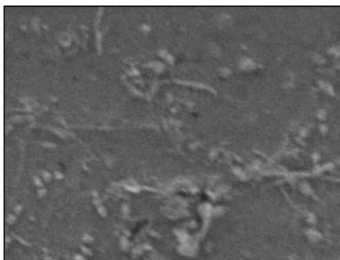
Fig. 5. SEM image of biofilm developed on surface of new pipeline made of PVC (magnification of 2 000 $\times$ )
