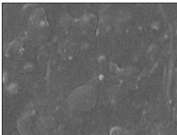
Fig. 12. SEM image of surface of new pipeline made of PP after biofilm removal (magnification of 1 800×)
