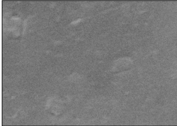
Fig. 1. SEM image of surface of new pipeline made of PVC (magnification of 6 000×)
