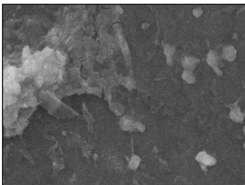
Fig. 6. SEM image of biofilm developed on surface of new pipeline made of PE (magnification of 2 000 $\times$ )
