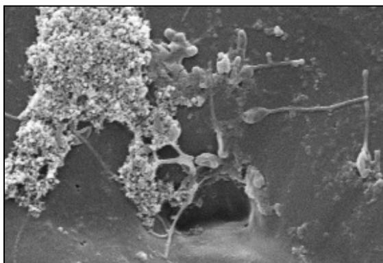
Fig. 8. SEM image of biofilm developed on surface of new pipeline made of PP (magnification of 1 500×)
