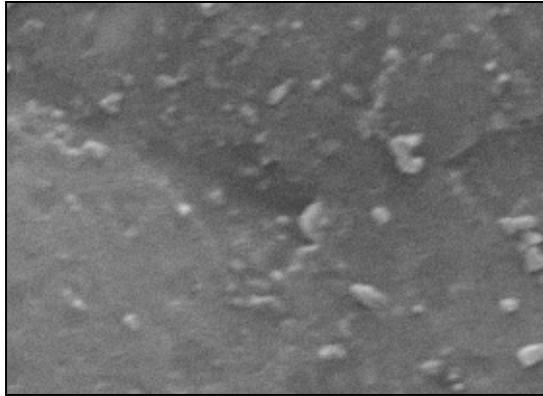
Fig. 3. SEM image of surface of new pipeline made of PB (magnification of 6 000×)
