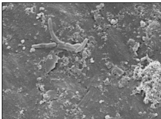
Fig. 11. SEM image of surface of new pipeline made of PB after biofilm removal (magnification of 1 800×)
