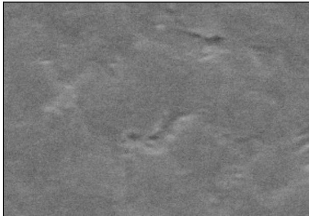
Fig. 2. SEM image of surface of new pipeline made of PE (magnification of 6 000×)
