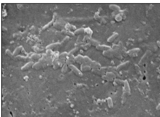
Fig. 7. SEM image of biofilm developed on surface of new pipeline made of PB (magnification of 1 800 $\times$ )
