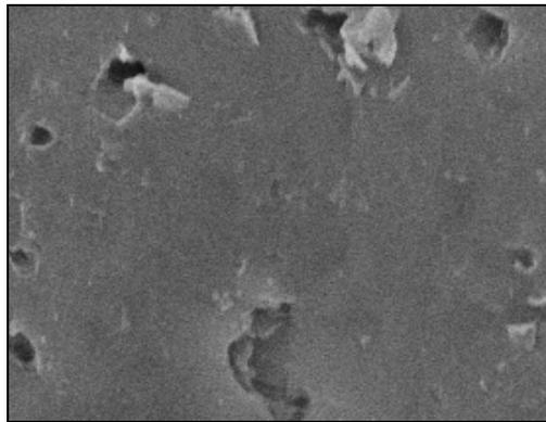
Fig. 9. SEM image of surface of new pipeline made of PVC after biofilm removal (magnification of 2 000 $\times$ )
