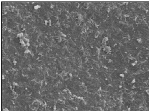
Fig. 10. SEM image of surface of new pipeline made of PE after biofilm removal (magnification of 2 000 $\times$ )
