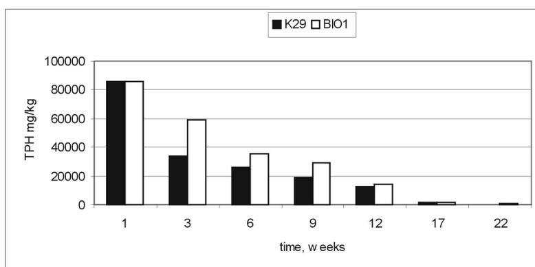
Fig. 1. Average concentration of diesel oil in soil from lysimeters
