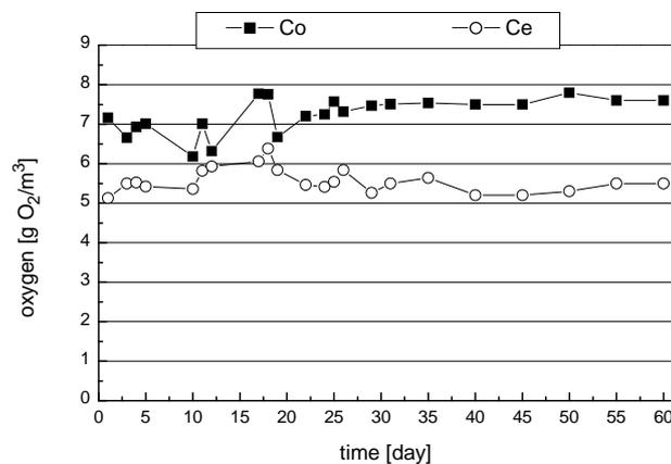
Fig. 4. Oxygen changes in raw water (Co) and the water treated (Ce) in diatomite bed
