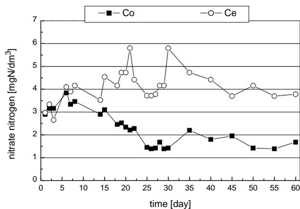
Fig. 3. Nitrate nitrogen changes in raw water (Co) and the water treated (Ce) in diatomite bed
