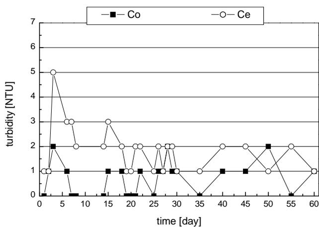
Fig. 6. Turbidity changes in raw water (Co) and the water treated (Ce) in diatomite bed
