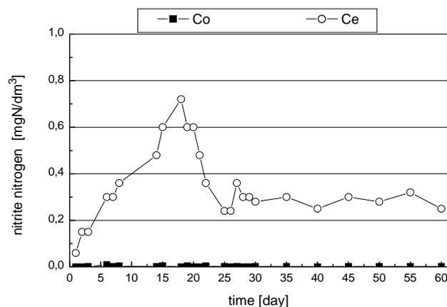
Fig. 2. Nitrite nitrogen changes in raw water (Co) and the water treated (Ce) in diatomite bed
