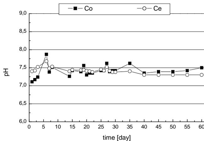
Fig. 5. pH changes in raw water (Co) and the water treated (Ce) in diatomite bed
