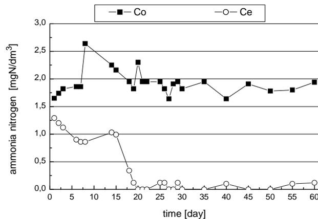
Fig. 1. Ammonia nitrogen changes in raw water (Co) and the water treated (Ce) in diatomite bed
