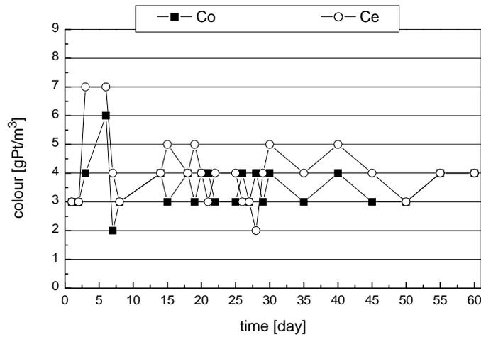
Fig. 7. Colour changes in raw water (Co) and the water treated (Ce) in diatomite bed
