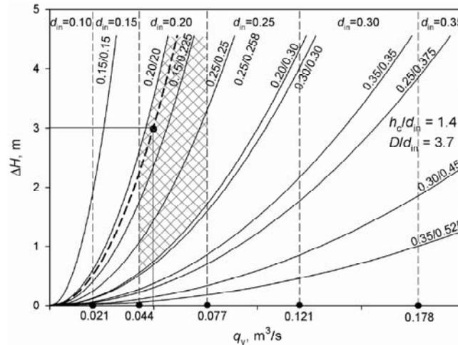
Fig. 9. The nomogram of hydraulic characteristics of cylindrical vortex regulators for the diameter relation  $d_{in}/d_{out}$  for  $h_c/d_{in} = 1.4$  and  $D/d_{in} = 3.7$  from range  $d_{out}/d_{in} \in \langle 1; 1.5 \rangle$  (for computational example)
