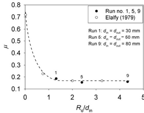
Fig. 5. The dependence of the coefficient  $\mu$  on the relation  $R_o/d_{in}$
