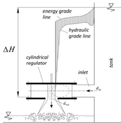
Fig. 1. Schematic diagram of cylindrical vortex regulator operation
