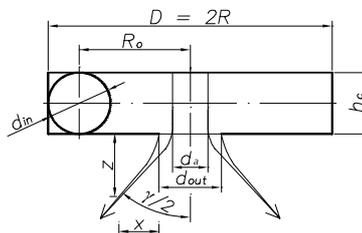
Fig. 2. Geometrical and operational parameters of vortex flow regulator
