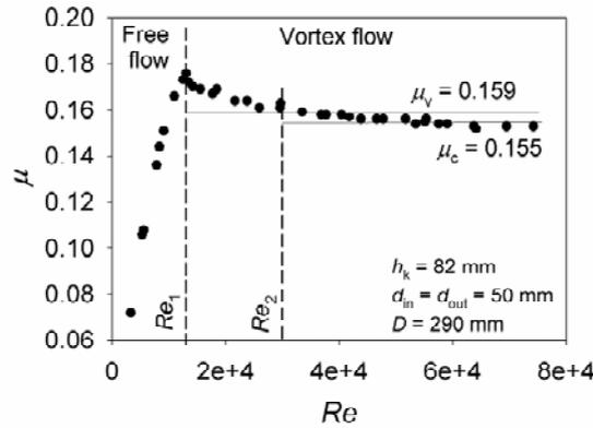
Fig. 4. The interpretation of the discharge coefficient values  $\mu_v$  and  $\mu_c$  above the boundary values of Reynolds numbers  $Re_1$  and  $Re_2$  for an example regulator
