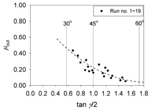
Fig. 8. The dependence of the coefficient  $\mu_{out} = \mu (d_{in}/d_{out})^2$  on  $\tan \gamma/2$  in vortex flow
