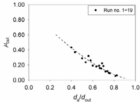
Fig. 7. The dependence of the coefficient  $\mu_{out} = \mu (d_{in}/d_{out})^2$  on  $d_a/d_{out}$  in vortex flow
