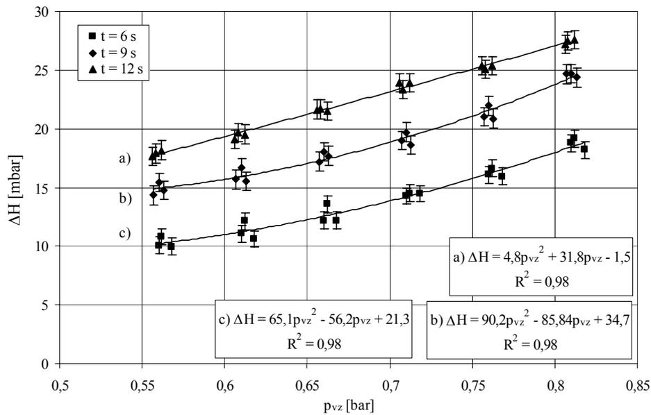
Fig. 3. Lift on the vacuum pipeline of 63 mm diameter
