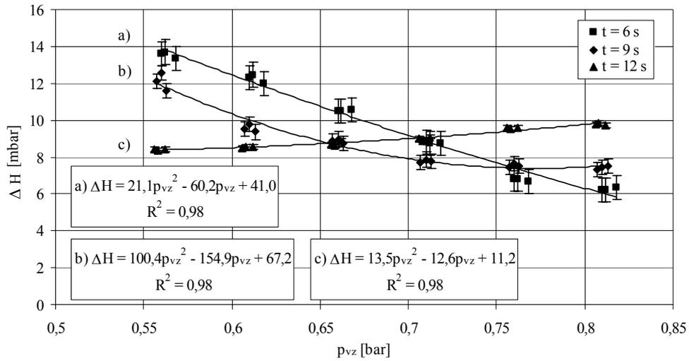
Fig. 5. Lift on the vacuum pipeline of 110 mm diameter
