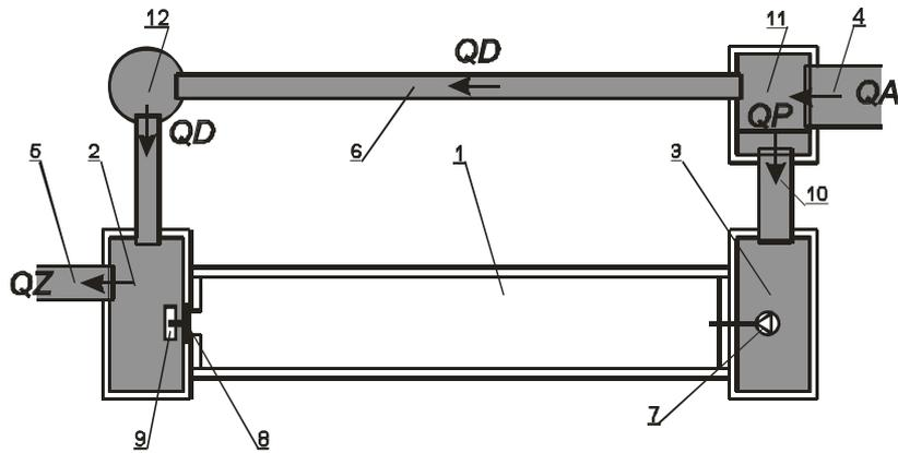
Fig. 3. *EcoINFRA2* storage reservoir functioning during the period of pump chamber filling
