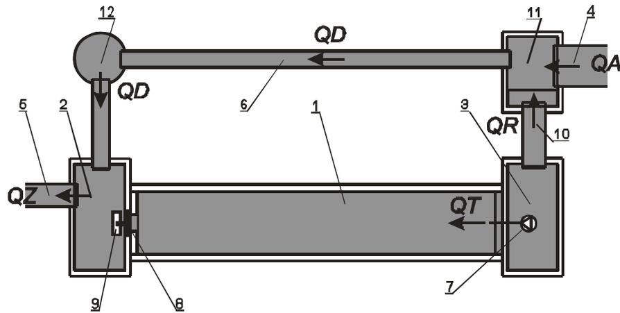
Fig. 5. EcoINFRA2 storage reservoir functioning during the period of emptying overflow and pump chambers
