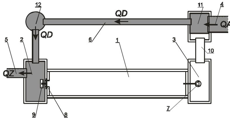
Fig. 2. EcoINFRA2 reservoir functioning during the period of dry weather
