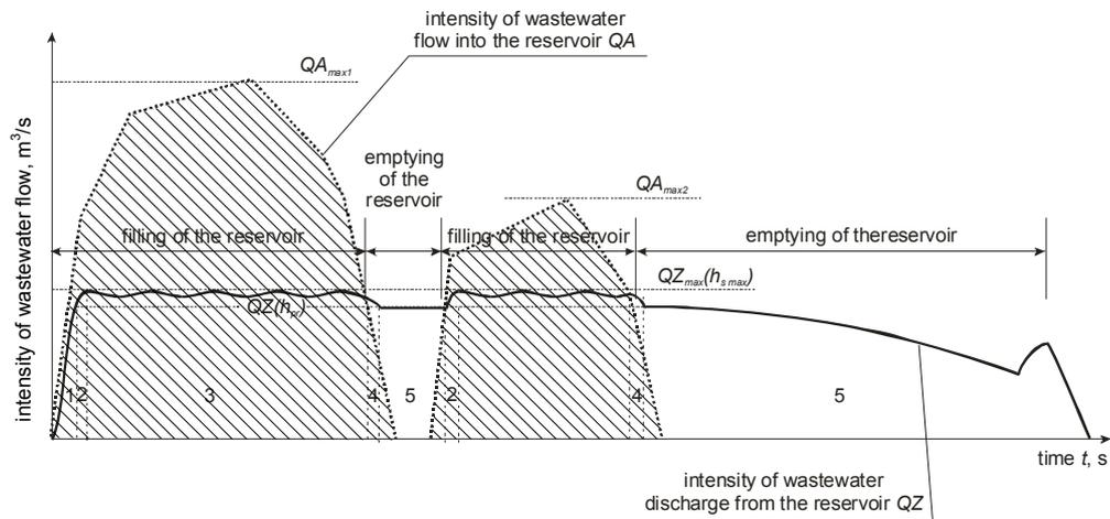
Fig. 8. Wastewater inflow and outflow hydrograms for *EcoINFRA2* storage reservoir during two successive rains in a short period of time (1 – filling of overflow and steering chambers, 2 – filling of a pump chamber, 3 – pump filling of an accumulation chamber, 4 – emptying of overflow and pump chambers, 5 – emptying of accumulation and steering chambers)
