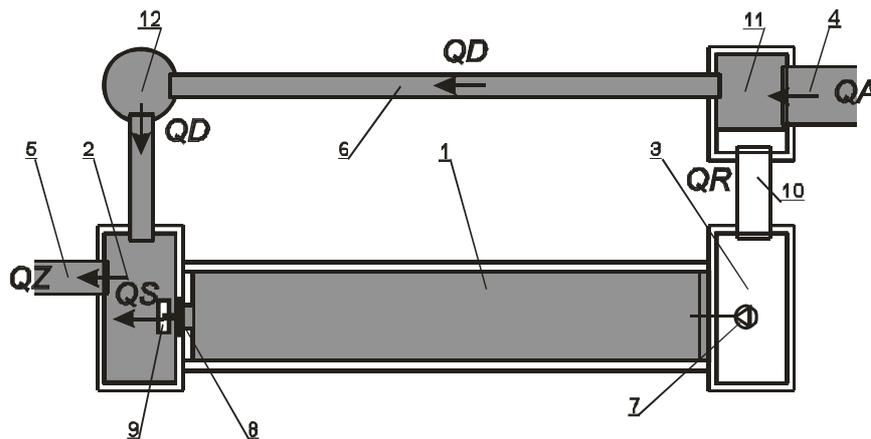
Fig. 6. *EcoINFRA2* storage reservoir functioning during the period of accumulation chamber emptying
