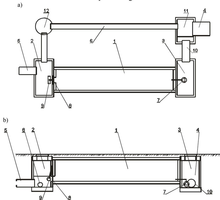
Fig. 1. *EcoINFRA2* storage reservoir hydraulic scheme: a) horizontal section of reservoir with choking pipe and inflow chamber; b) vertical section of reservoir with choking pipe and
