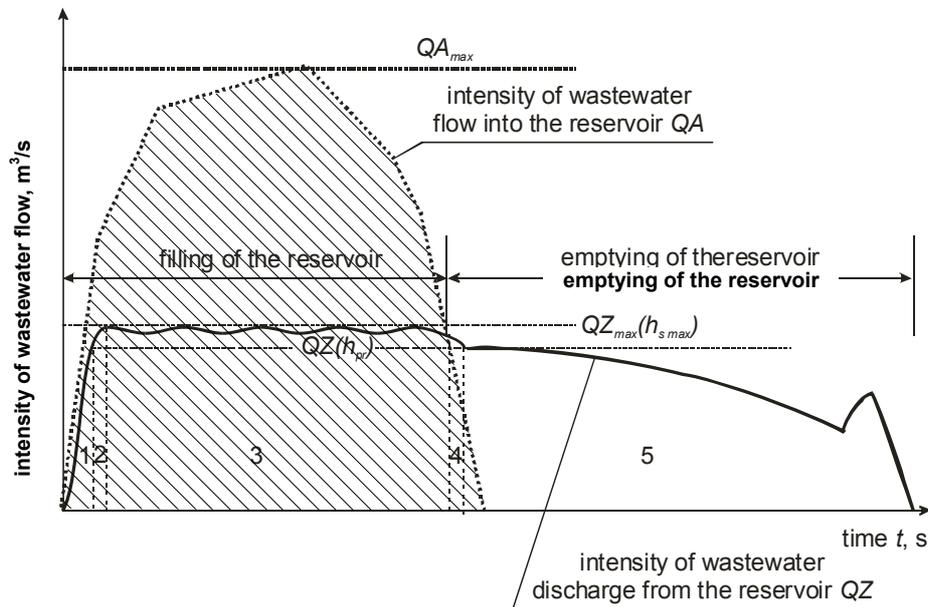
Fig. 7. Wastewater inflow and outflow hydrograms for *EcoINFRA2* storage reservoir in the case of intermittent rain (1 – filling of overflow and steering chambers, 2 – filling a pump chamber, 3 – pump filling of an accumulation chamber, 4 – emptying of overflow and pump chambers, 5 – emptying of an accumulation and steering chambers)
