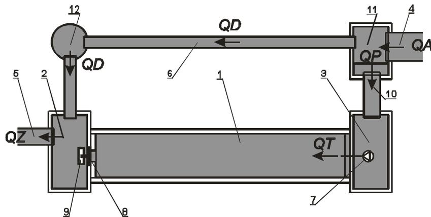
Fig. 4. *EcoINFRA2* storage reservoir functioning during the period of accumulation chamber filling
