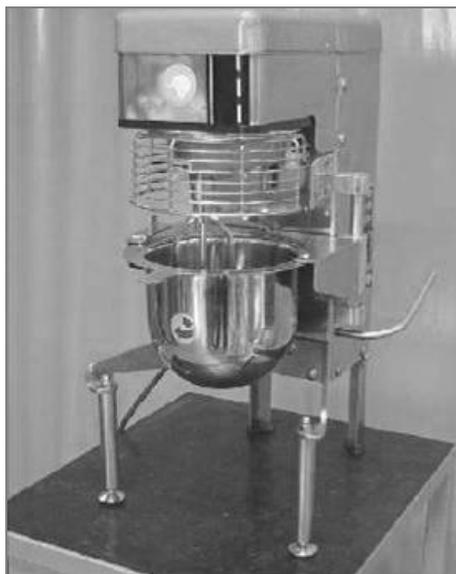
Fig. 1. Mixer for cement mortars, Tecnotest B205/X5
