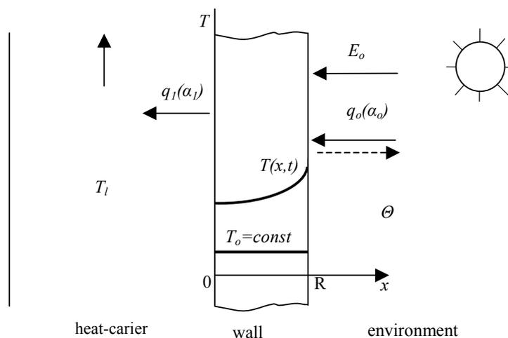
Fig. 1. The scheme of heat interchange in the collector wall
