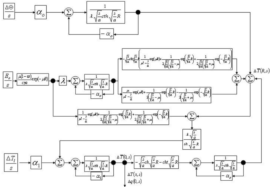
Fig. 2. Structural scheme of the solution of the equation for the plate thermal conduction
