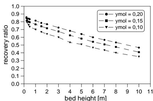
Fig. 2. Influence of bed height on recovery ratio
