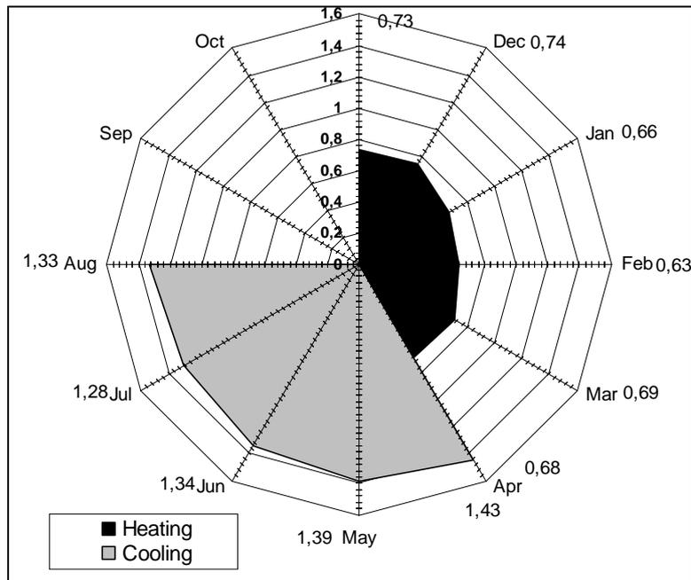
The efficiency of air-split heat pump: heating and cooling [1], [2]
