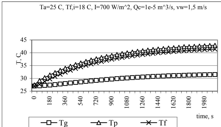
Fig. 1. Heating characteristics of the solar collector as a function of time
