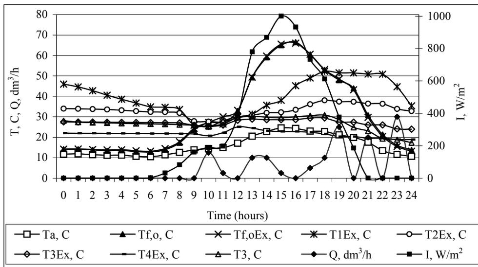
Fig. 3. Heating the working medium in the SDHW system
