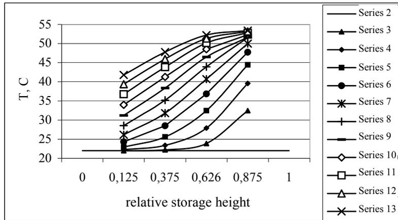
Fig. 2. Distribution of temperature in the storage tank during loading phase
