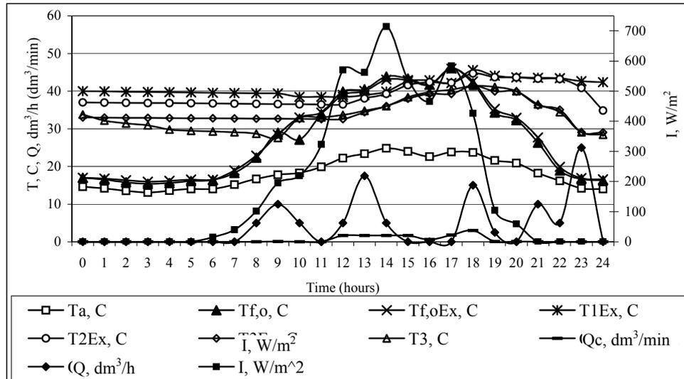
Fig. 4. Heating the working medium in the SDHW system in comparison with external inputs
