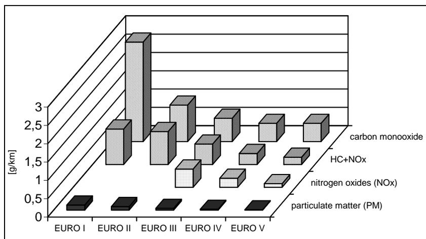
Fig. 2. Increasingly stringent emission standards for cars and LDV with Diesel engines
