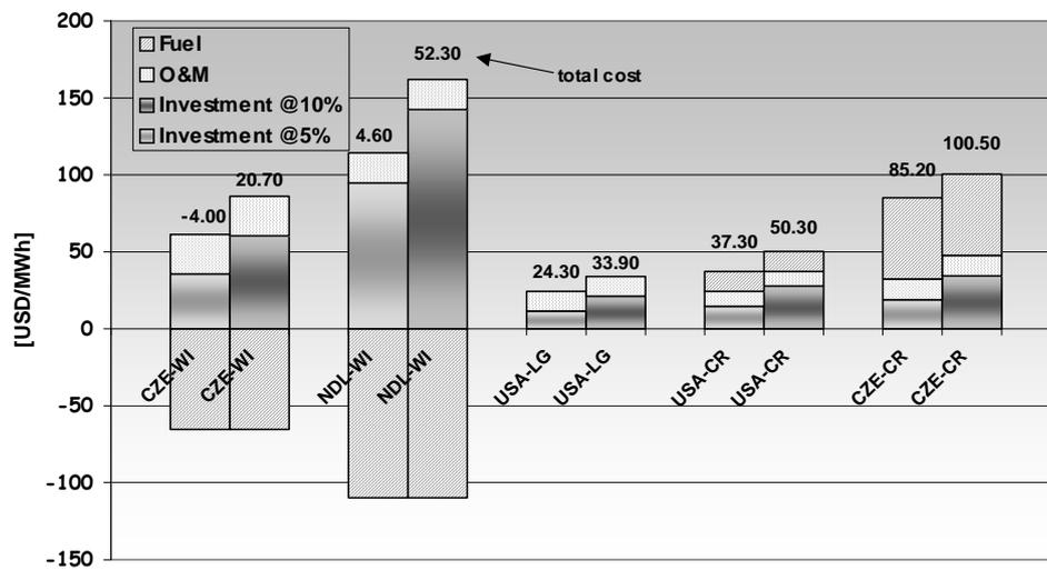
Fig. 1. Cost of electricity from biomass-fuelled generation plants
