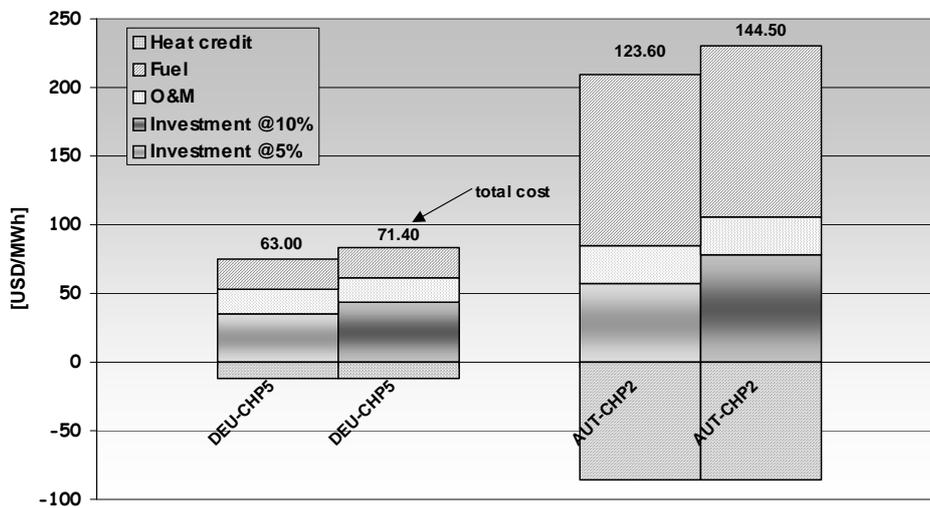
Fig. 2. Cost of electricity from biomass-fuelled thermal-electric power stations
