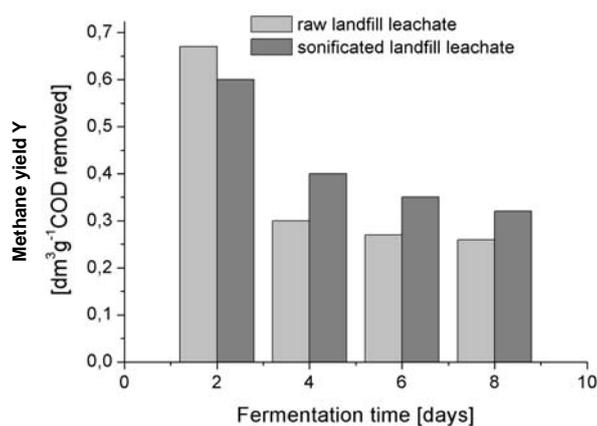
Fig. 5. Methane yield versus fermentation time for raw and ultrasonicated landfill leachate
