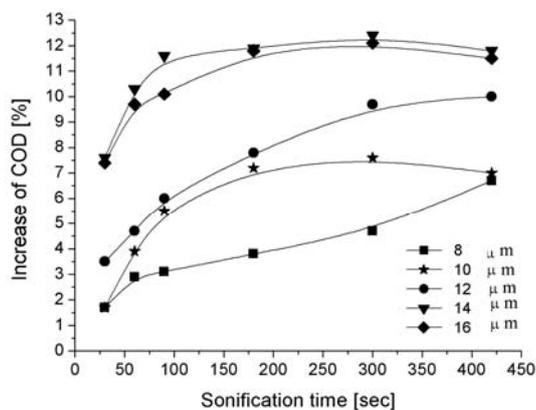
Fig. 2. An increase in COD in landfill leachate versus amplitude of ultrasonic field and the time of ultrasonication
