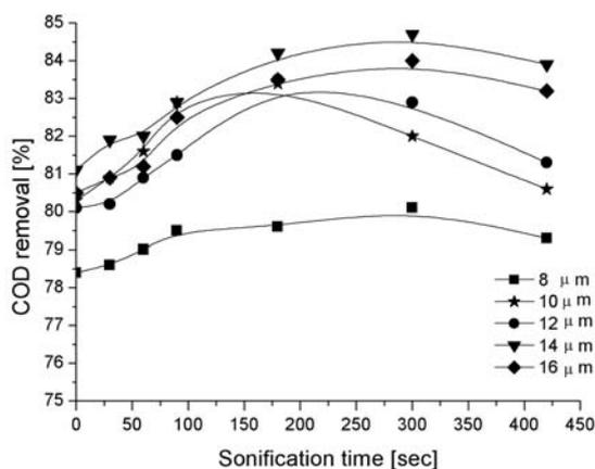
Fig. 3. Ultrasonication time and amplitude versus COD removal
