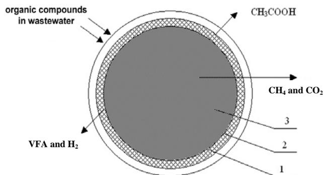
Fig. 1. Structure of anaerobic sludge granule [7]:
