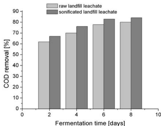
Fig. 4. Comparison of COD removal efficiency during fermentation process of raw and ultrasonicated landfill leachate
